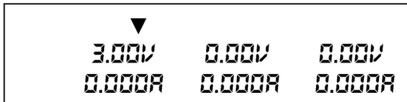
Figure 9 – VFD display: Outputs of Power Supply disabled. Channel 1 selected.
